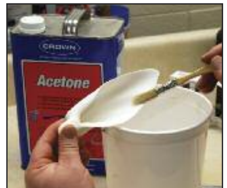
Clean the liner with acetone and let it dry.
